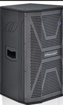
Cx. Passiva 2 Vias, c 01 A.F 10" + Driver TI , Conector Speakon/P10, (SPL MAX CONTINUO Campo Livre 111dB / SPL MAX PICO Plano Terra 129dB).
