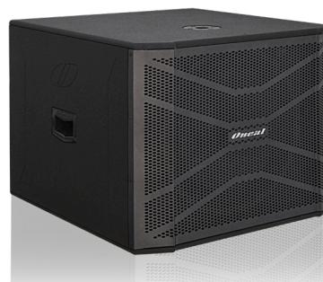
Cx. Ativa Bass Reflex "Outback", c/ 01 A F 12" , 04 Ohms, cor preta, Resposta 30/480Hz e CFA 95 Hz a 480 Hz, ICS/ARP/SCP/ETP/CLP/BI/PHI/SPOT/Chave Lift Gnd 110/220Vac, (SPL MAX CONTINUO Campo livre 111,0dB / SPL MAX PICO Plano Terra 129,0dB)
